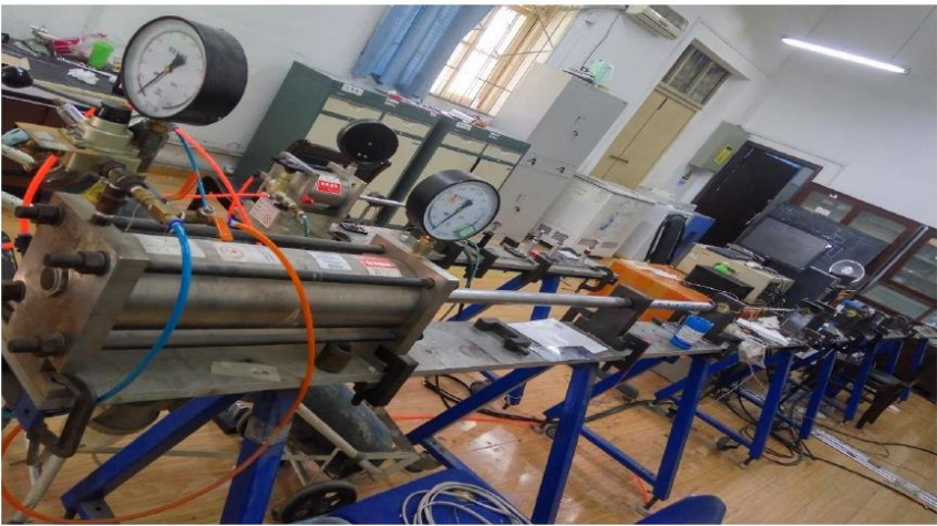
Figure 2: Split Hopkinson Pressure Bar (SHPB)[2]
